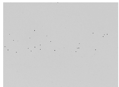
Fig. 2: Tracks of the fission products on our Boron-coated plastic detectors
